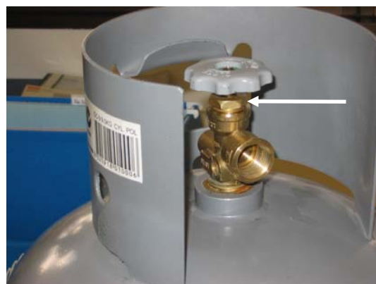
Valve showing loose gland nut
