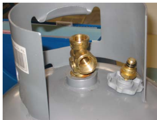
Valve can fall apart during closing action
